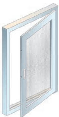
Hinged windows can open inward or outward.
