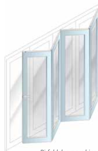
Bi-fold doors are hinged to fold neatly to one side in a concertina style.
